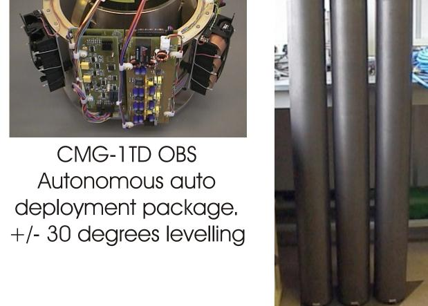
CMG-3ESPD Compact OBS. 24-bit ADC. +/- 10 degrees leveling Titanium housing
