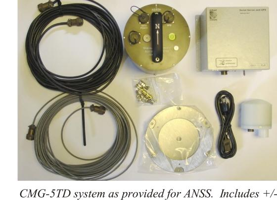
4g > 145dB accelerometer, 24-bit digitizer with flash memory, baseplate for fixing and UPS with TCP/IP serial server communications
